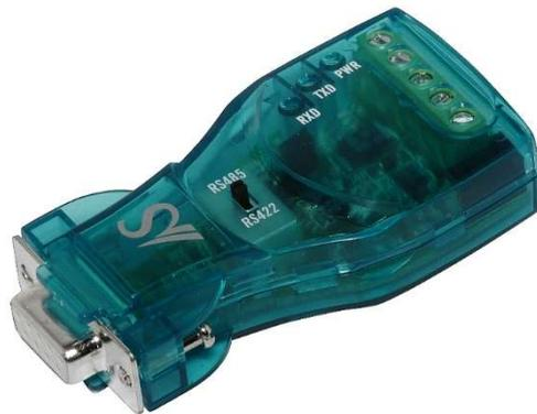
CS-428/9AT-PRO2 converts RS232 signals to RS422 or 485. It is an efficient solution for applying advantages of RS422/485 to legacy RS232 devices. The converter operates with no extra software installation, and with simple DIP switch toggling, RS422 or RS485 can be selected. Also, the product is fully compatible with serial COM port in PC.
