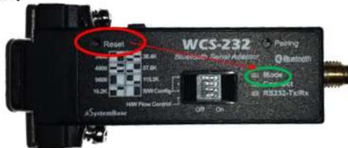
Press the Reset button on #4 for more than 2 seconds.
