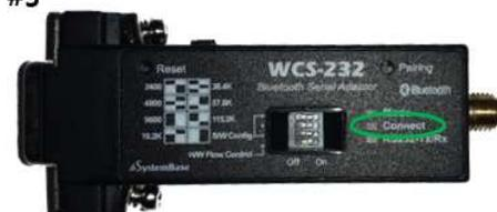
The Connect LED of the connected #1(main), #2, #3, #4 and #5 flashes.
