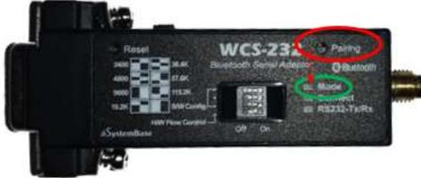
Press the Pairing button on #1(main) for more than 2 seconds.
