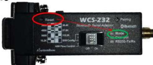
Press the Reset button on #3 for more than 2 seconds.
