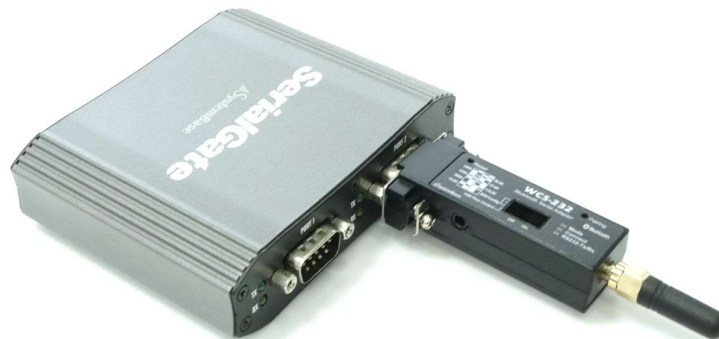
[Figure 0-3 Connecting WCS-232 to a serial device]
