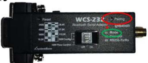
Press the Pairing button on #5 for more than 2 seconds.
