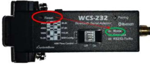
Press the Reset button on #5 for more than 2 seconds.
