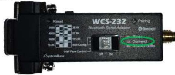
The Connect LED flashes. You can change the serial port speed after, according to the switch diagram.
