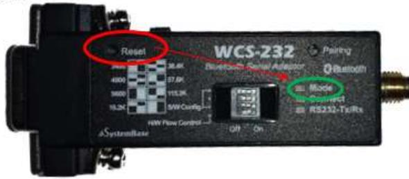
Press the Reset button on #2 for more than 2 seconds.
