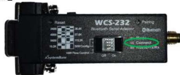
The Connect LED of the connected #1(main) and #2 flashes.
