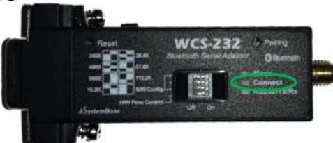
The Connect LED of the connected #1(main), #2 and #3 flashes.
