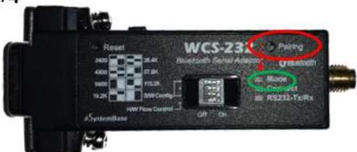
Press the Pairing button on #4 for more than 2 seconds.
