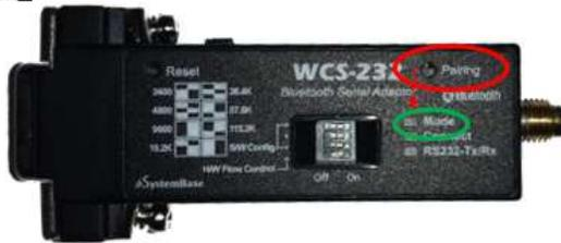
Press the Pairing button on #2 for more than 2 seconds.
