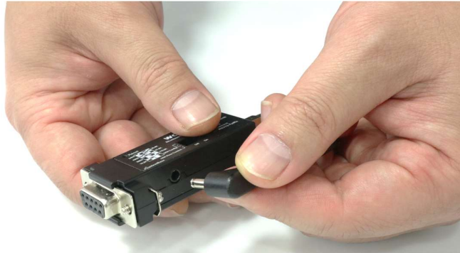
[Figure 0-2 Connecting power to WCS-232]
