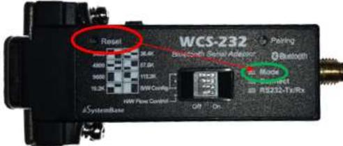
Press the Reset button on #1(main) for more than 2 seconds.
