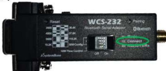
The Connect LED of the connected #1(main), #2, #3 and #4 flashes.
