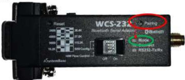
Press the Pairing button on #1 for more than 2 seconds.
