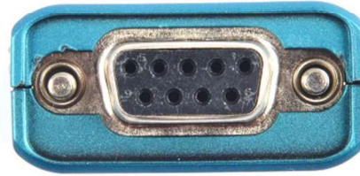
Serial Port(RS232/RS422/RS485)
