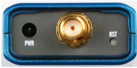
DC Adapter, LoRa Antenna Connector
